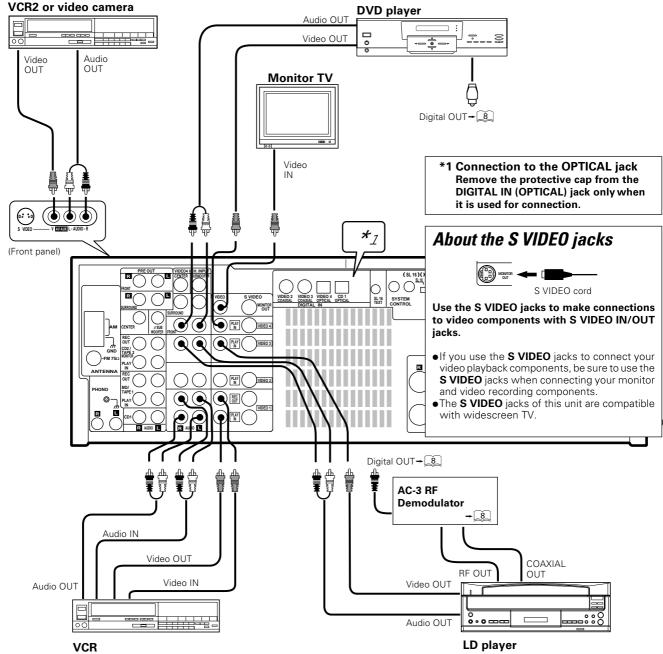
• To connect a Video CD compatible CD player and outputs its video, connect the player to one of the sets of input jacks **VIDEO1** to **VIDEO4**. In this case, do not connect the system control cord to the CD player.
